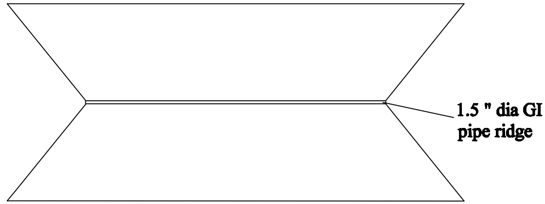
Top of roof
